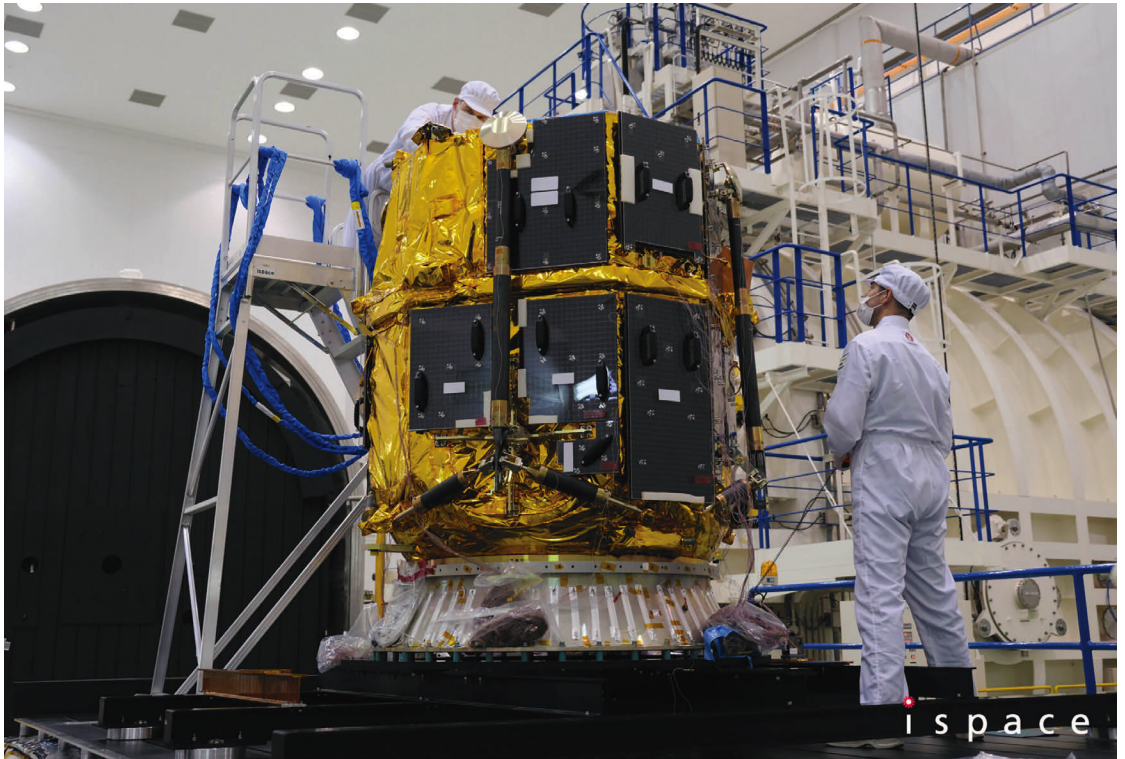
Right: Resilience, the second ispace lunar lander, recently completed environmental testing ahead of a launch scheduled for late this year.
